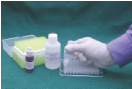
1. Add 5 drops of sample diluent to the first row of wells on a microtiter plate.
