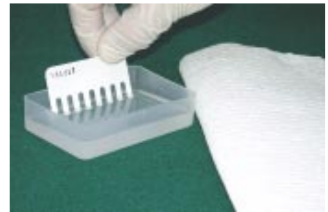
6. Dilute the rinse buffer 5-fold in a tray and wash comb. Allow to drain as in Step 5.
